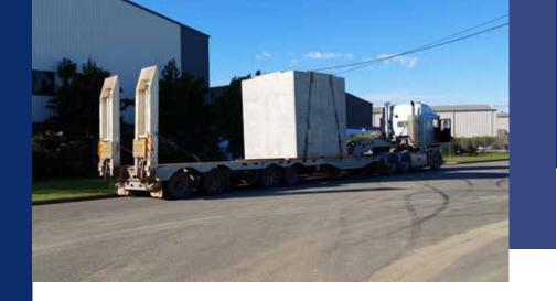
Two lift shafts were manufactured for the project, in a Class 2 off-form finish with chamfered edges.
