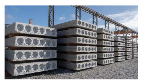
Using hollowcore also dramatically improves construction speed and makes sites safer by reducing clutter and activity on site and transferring works to a controlled factory environment.
