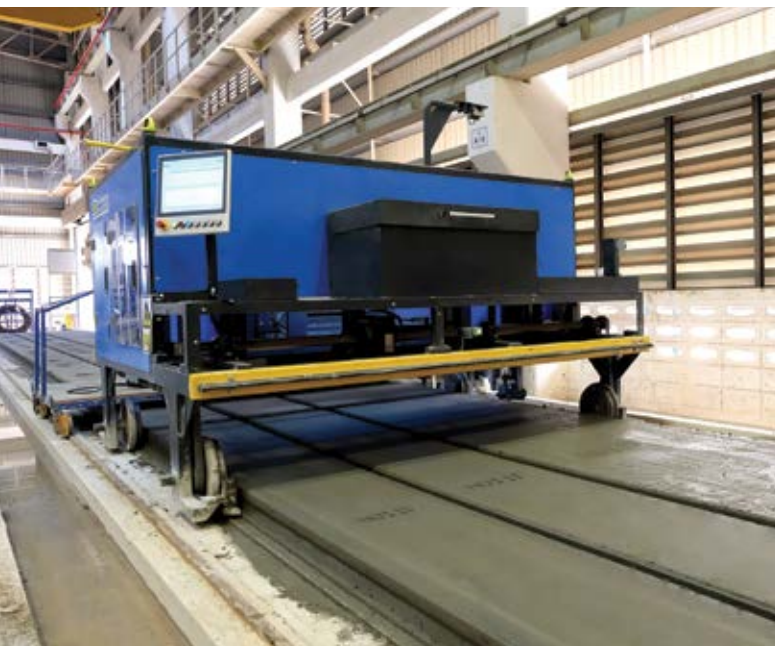
ABOVE (L&R): The SamrtJet automatic plotter works with the CAD data imported through the EBOS HC software. This machine ensures fast marking on the slabs, with no mistakes made. The markings for the Line Detection are made simultaneously.
