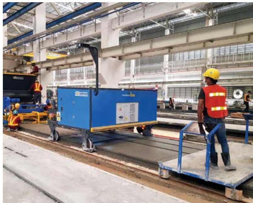
ABOVE (L&R): The SamrtJet automatic plotter works with the CAD data imported through the EBOS HC software. This machine ensures fast marking on the slabs, with no mistakes made. The markings for the Line Detection are made simultaneously.
