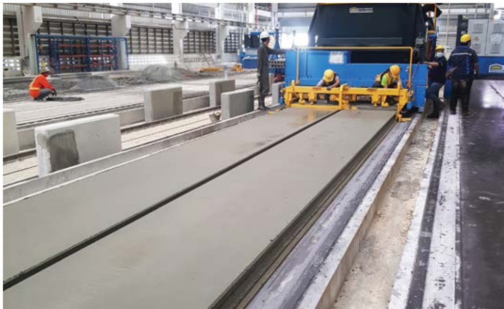
ABOVE & TOP: The Slipformer S-Liner is a flexible machine. It is capable of producing 1 slab 1.2m in width and 2 slabs of 0.6m, or two slabs of 1.2m at the same time.
