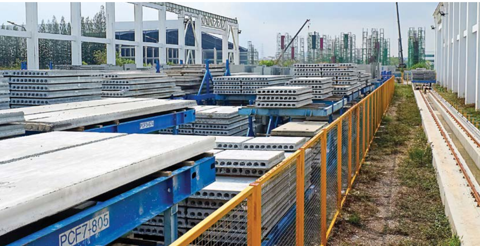
ABOVE: The highly automated Pruksa plants produce hollow core slabs for use in sustainable residential and commercial buildings.
