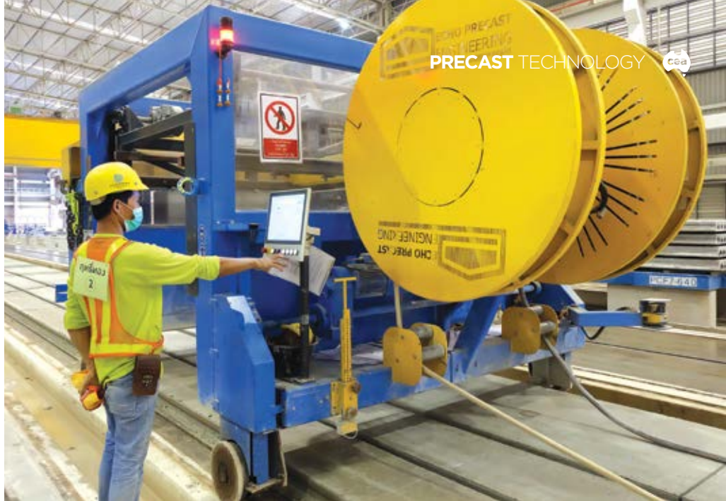
ABOVE: The fully automatic Multi Angle Sawing Machine (MAS) incorporates an array of safety sensors for a safe environment. The unit can function in fully-automated mode using Echo Precast Engineering's patented 'Line Detection' technology.
