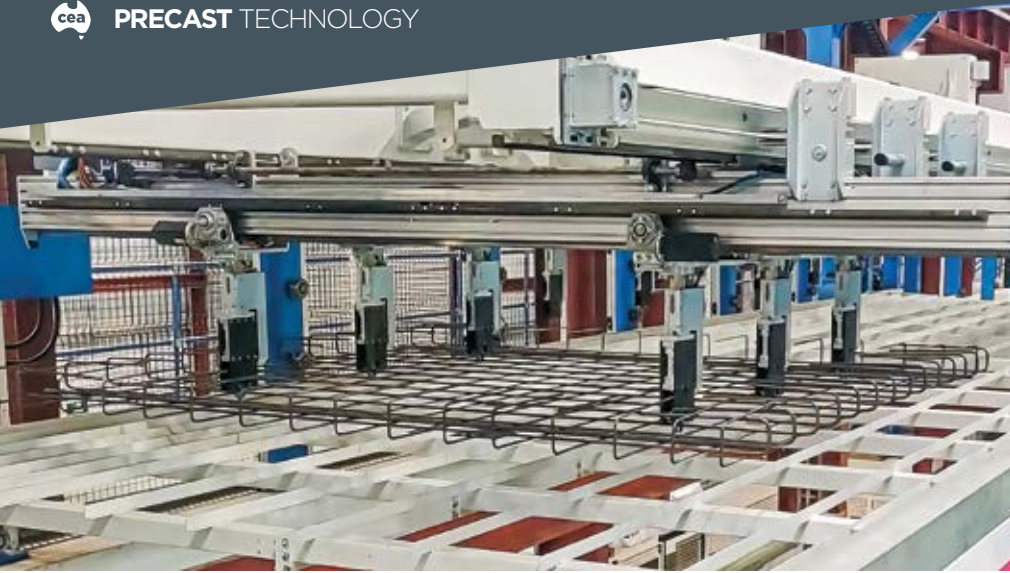
LEFT: The innovative traverse gripper automates the logistics process even for specially bent mesh and cages.
