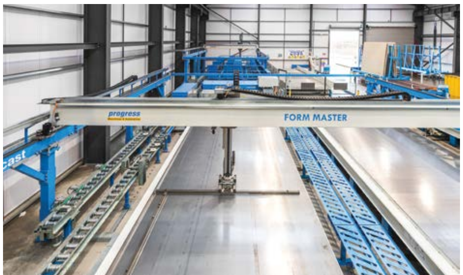
ABOVE: The Form Master shuttering robot places the shutters automatically and precisely on the pallet surface, without the need for filling elements that would have to be disposed of afterwards.
