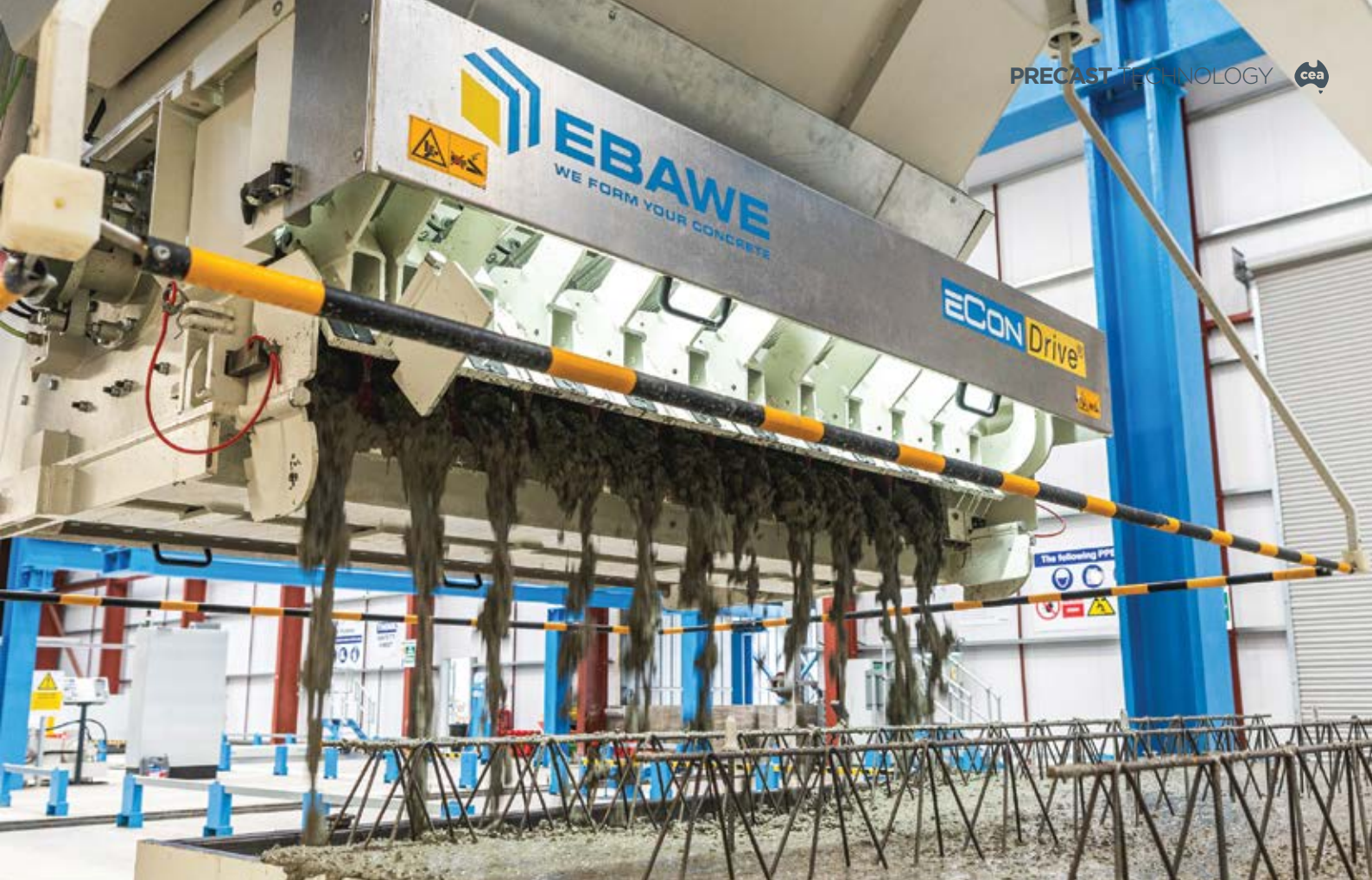
ABOVE: With the automatic eCon Drive® concrete spreader connected to the plant's high-tech software solutions, the amount of concrete spread is calculated accurately, thereby reducing waste.
