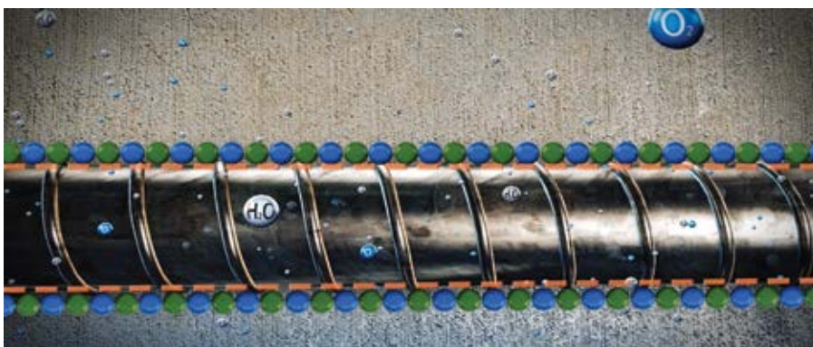
A conceptual illustration of how Migrating Corrosion Inhibitors create a molecular barrier against corrosion on the surface of embedded rebar.. Image courtesy Cortec Middle East
