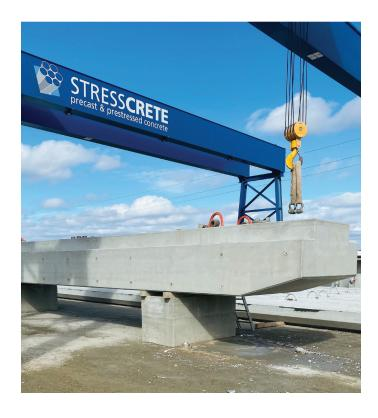
factory-controlled environment, the typical congestion of trades and materials deliveries is reduced on the construction site. The offsite manufacturing process allowed Stresscrete to deliver precast elements with consistent strength and finish quality across the entire project. When using precast concrete, the reduced congestion of onsite labor makes better access to the construction site and regulated precast factories can ensure the safest possible working conditions.
