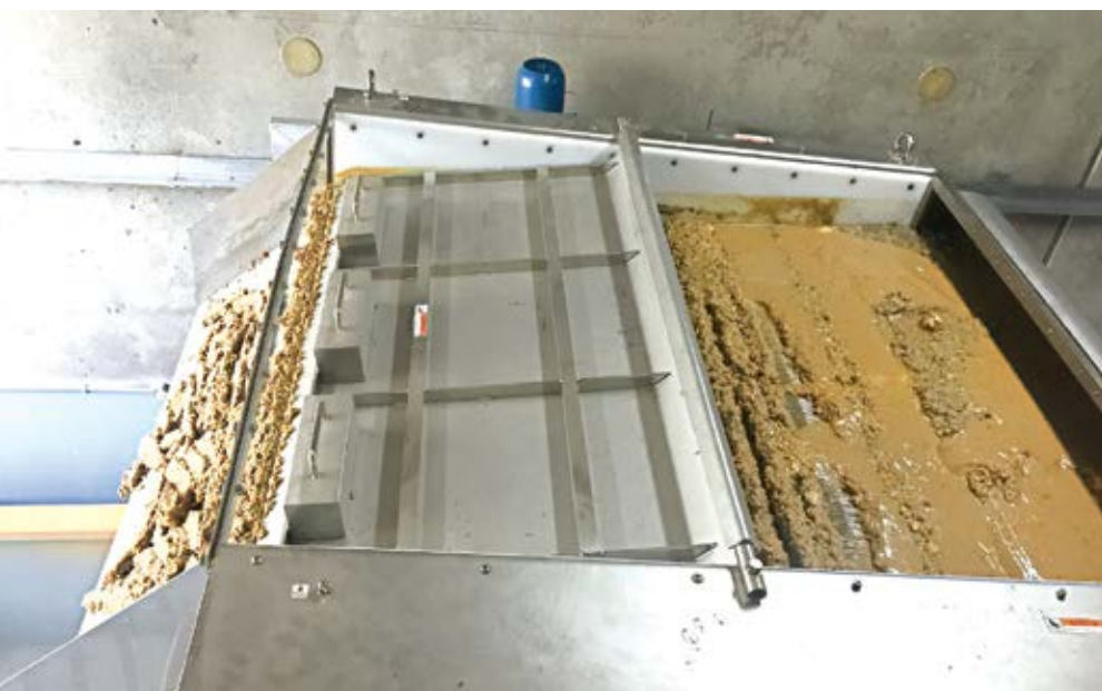
Heavy, sloppy food waste pulp going into the KDS solid-liquid separator (right) emerges as lighter, drier, more hygienic and more easily transportable waste cake (left).
