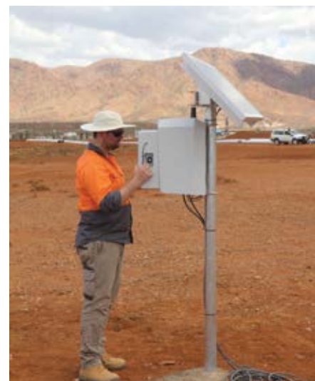
SENSEI is an autonomous off-grid system which delivers continuous data streams from remote locations. Powered by a solar panel, the data is transmitted via an internet connection direct from the source and into the digital cloud, giving user the ability to access and analyse the information on-site or from farther afield.
