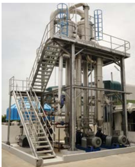
Evaporation and concentration systems based on heat exchangers have a small footprint, making them ideal for decentralised water treatment.
