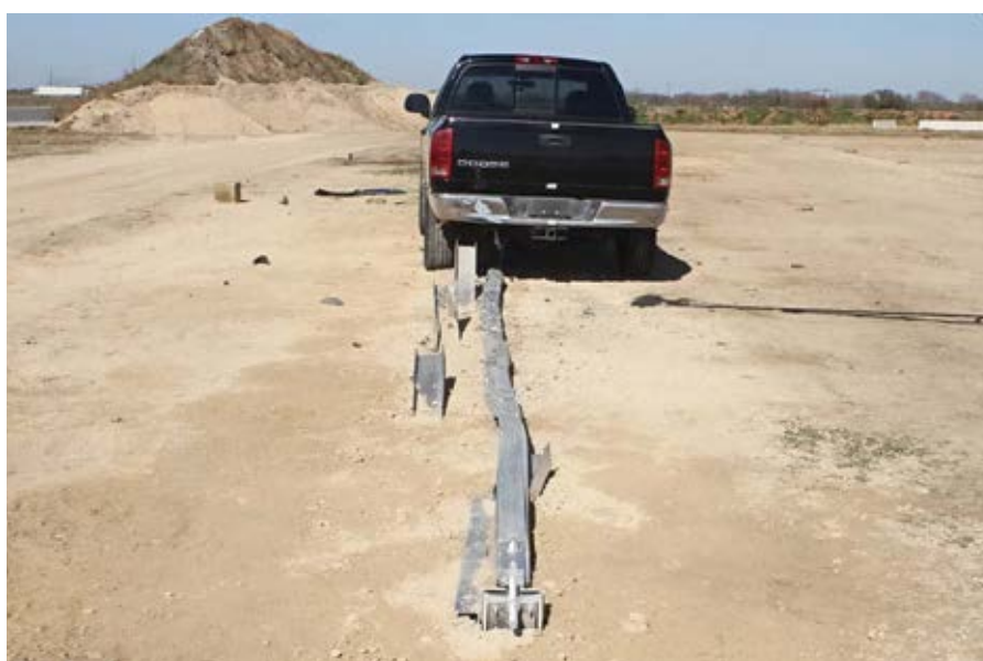
MASH TL-3 capacity end-on test with guardrail remaining anchored after impact
