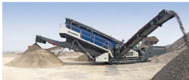
Screening plants like the MOBISCREEN MS 953 EVO screen the milled material to achieve an optimum PSD curve, making it possible to increase the amount of RAP added to the asphalt mix.
