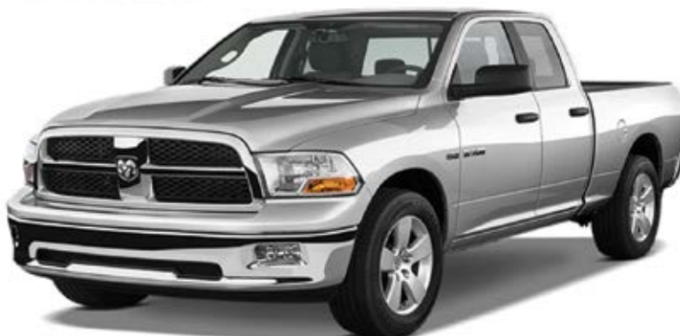
Below: The weight of large vehicle (pickup truck) used in TL3 containment testing was increased from 2000kg up to 2270kg.
