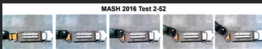
TMA alone is capable of absorbing the energy of the impact without having to rely on the host-vehicle rolling forward, it also means that the Scorpion II® Metro TMA is the only TL-2 TMA to be MASH certified with no upper weight limit for the host vehicle."
