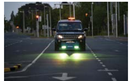
The RetroTek-D vehicle mounted retroreflector can operate day or night and check the condition of line markings on both sides of the lane at the one time.
