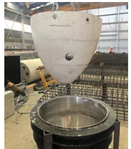
A Class 2 finish was required finish for the curved radiused sections of the mast and capping sections
