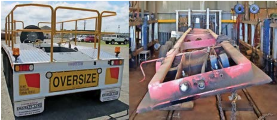
Chassis Line's experience ranges from new vehicle manufacturing, such as the trailer (left), through to repairs, servicing, modifications, safety assessments, and chassis straightening (right) - extending even to twisted chassis such as this example, which was damaged in a rollover.
