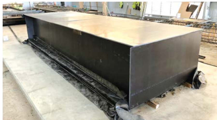
Top: Steel moulds were custom manufactured to cast the elements.
