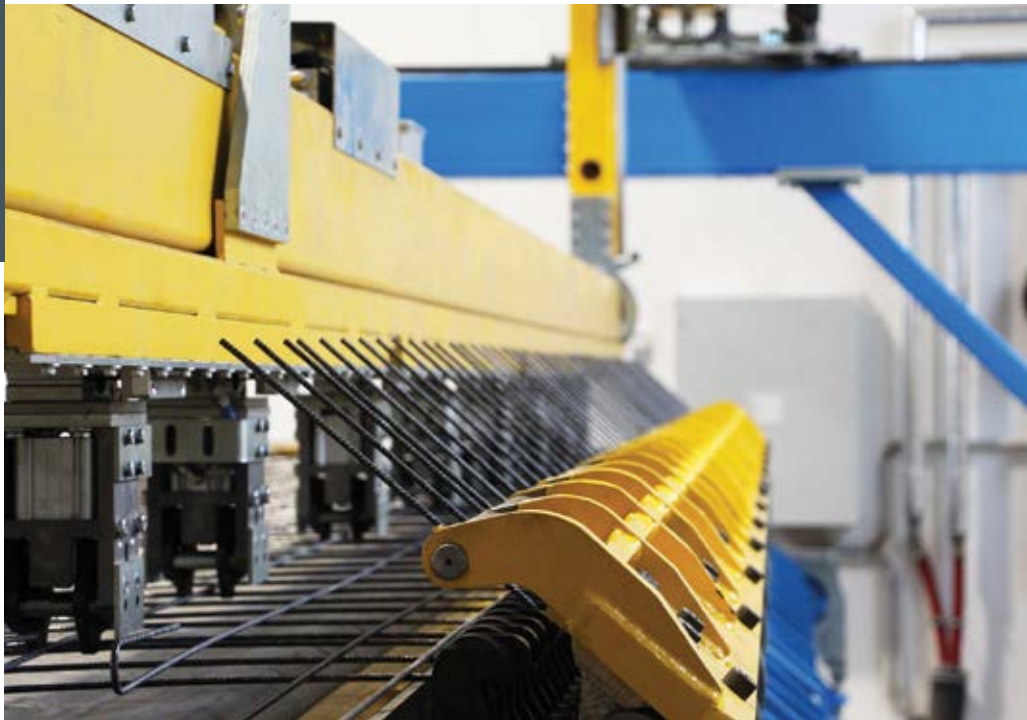
ABOVE: Beam bender in operation manufacturing bent end products automatically.
