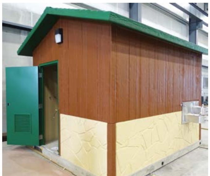
Huffcutt manufactures sanitary houses from solid concrete elements and assembles them directly in the plant, already completed with all sanitary facilities. The small buildings feature designs which utilise coloured concrete and form liners in tile, stone and wood optics.
