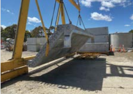
Custom wave generation components for Waveswell Energy to generate power off King Island, TAS (Hudson Civil Products)
