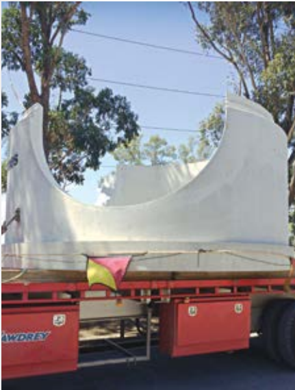
Pump-well pits for Westconnex, Kingsgrove, NSW (Humes)
