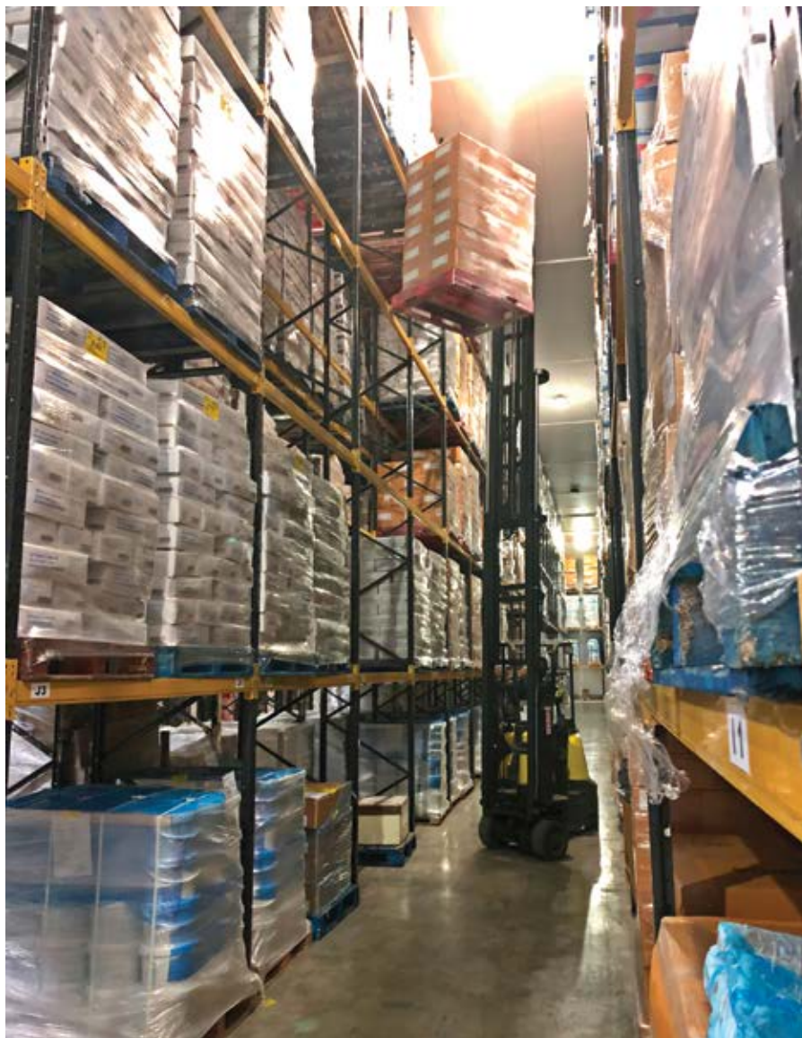
Combilift forklifts and stackers only requires around half the aisle space of a standard forklift to operate, allowing for a significant reduction in aisle widths.
