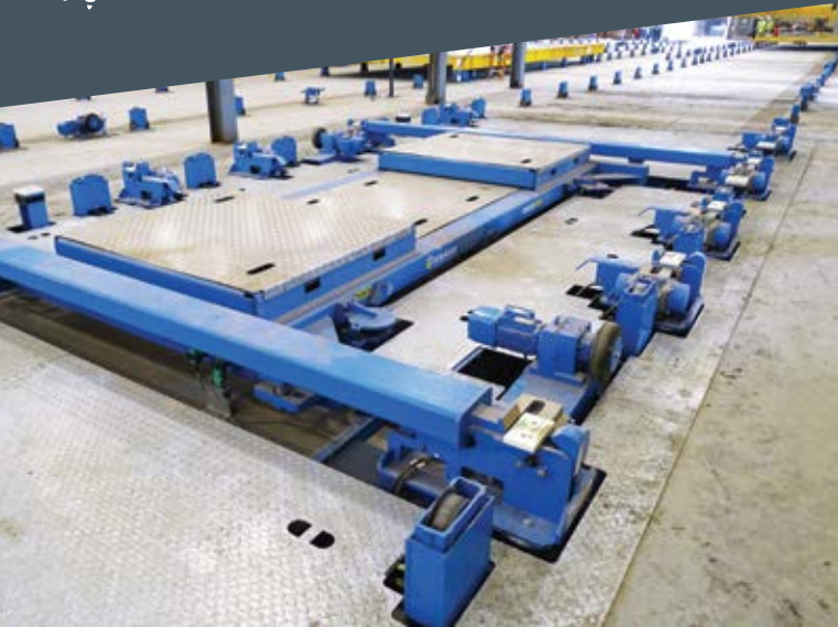
The combined compaction equipment moves the pallet vertically and horizontally, giving the customer maximum flexibility in the final product.
