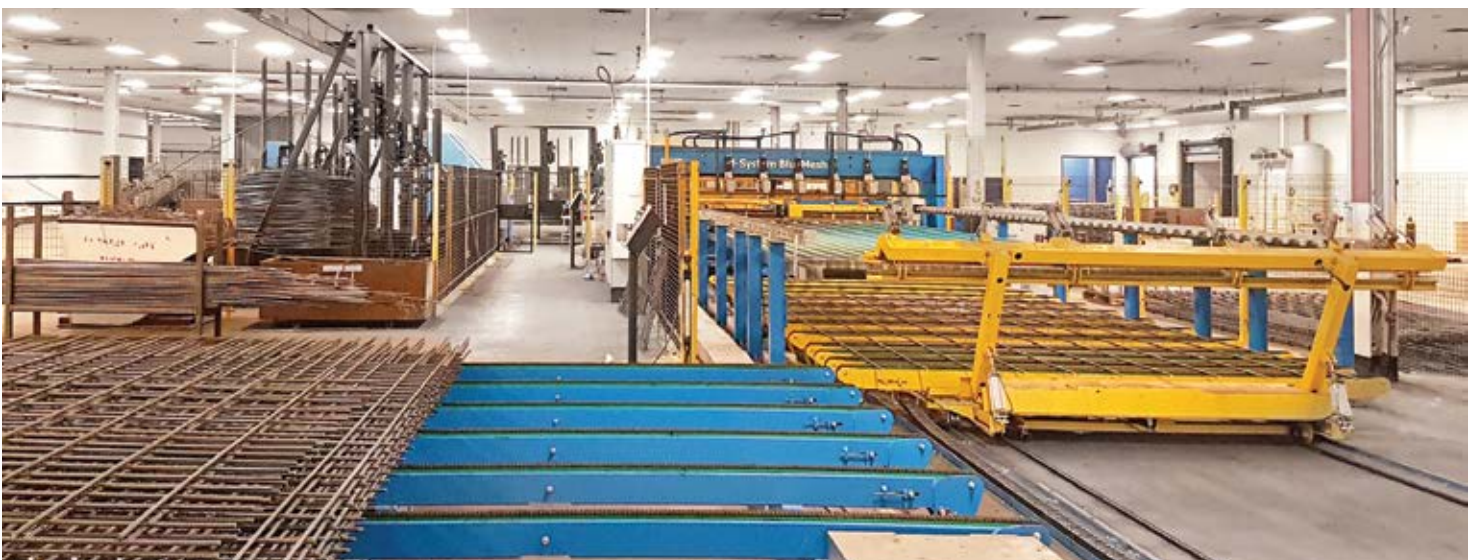
Below: The mesh welding machine M-System BlueMesh is a flexible production plant for welding bespoke mesh from coil according to individual specifications for each solid wall.
