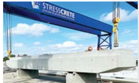
One of 7, 70 tonne, 13 metre headstock units for Smithfield Bypass, Cairns QLD (Stresscrete)
