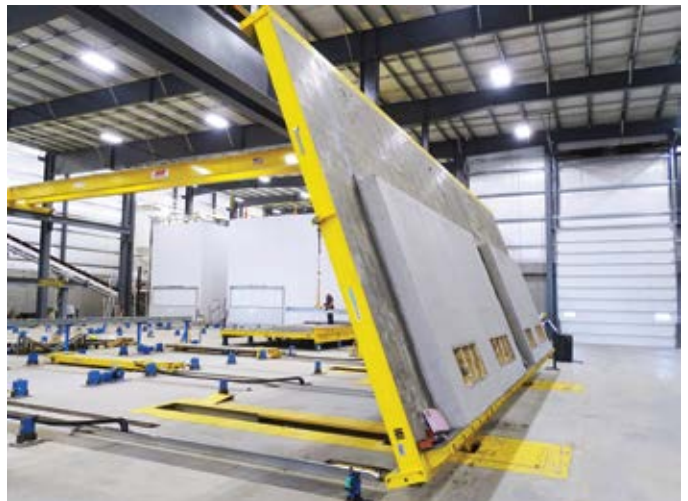
With the aid of the tilting device, the wall elements are tilted and can be conveniently stored in the subsequent installation position.
