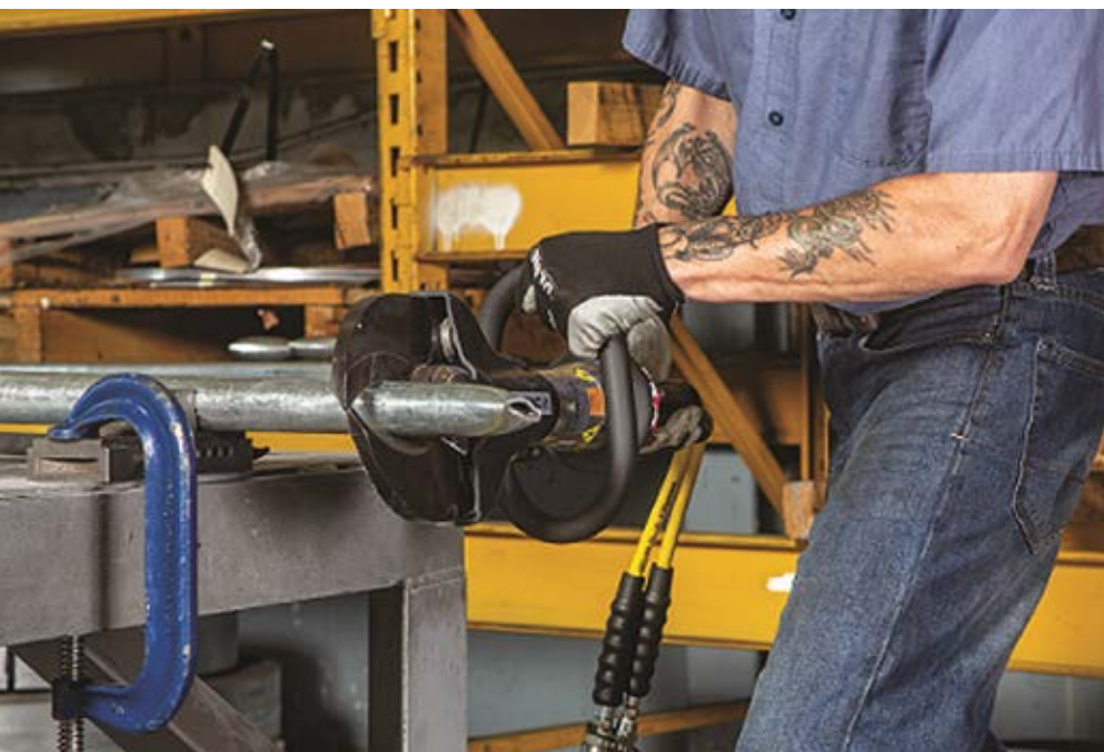
The purpose-designed EDCH Series 700 bar hydraulic cutters – which feature exceptionally large blade apertures, up to 170mm – can handle material hardness of up to 41HRc (Rockwell measure), including metal tubes, cables, profiles and similar materials.
