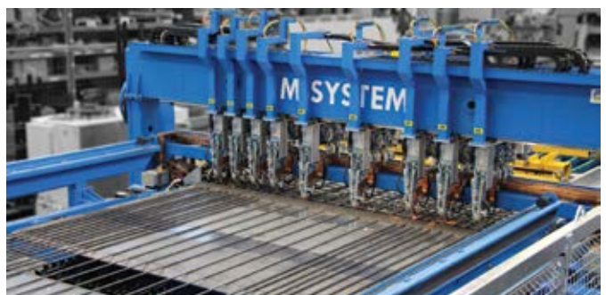
The M-System: Precise welding and made-to measure mesh production.
