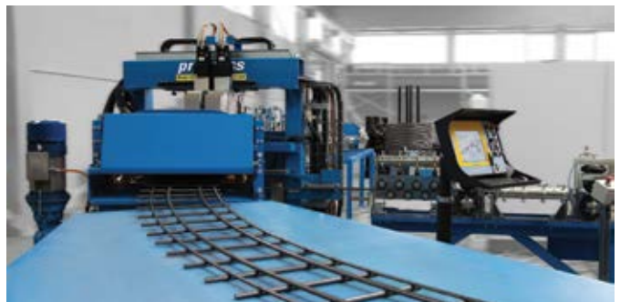
The Tunnel Master welds straight and bent ladders off coil.
