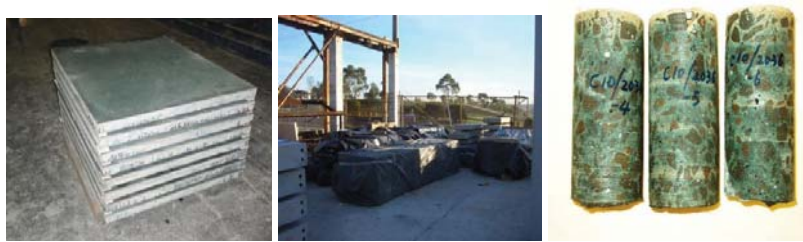
Fig. 3. Storage/ curing of precast geopolymer footway panels and geopolymer concrete cores with distinctive green colour
