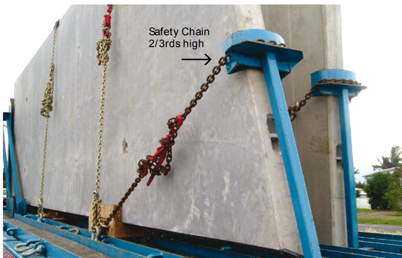
Figure 4, Restraining panels on a rear-tilt frame on a flat top trailer.
