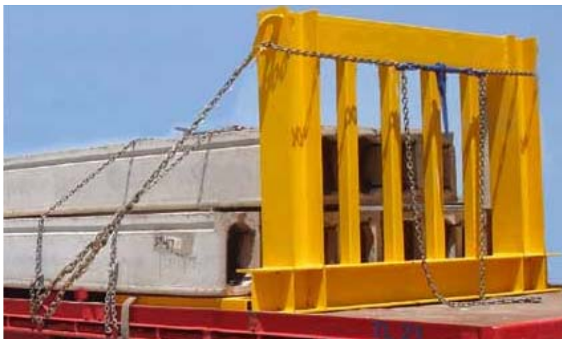
Figure 5, An example of a frame at the front of flat panels. "Safety Chain" around the blocking frame as well as the load resting on the frame base.
