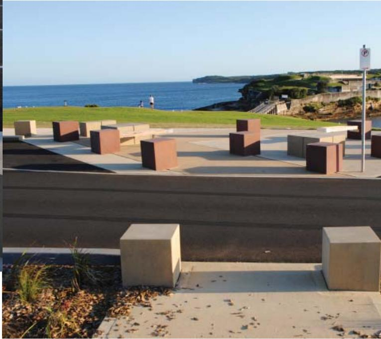
The highly corrosive coastal environment created by salt spray required careful consideration of materials, with concrete the obvious choice in terms of its impressive durability and minimal maintenance. The choice was the use of nearly 600 elements in five different shapes - wheel stops, separation blocks, kerbs and two styles of bollards that provided a 'garrison look' to the project.
