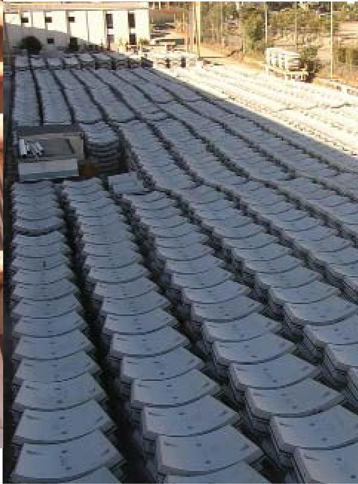
Director Ian Coulter says precast concrete was chosen to ensure reliable delivery, easy segment installation and a high quality finish. “We had to specially manufacture a huge 22,000 concrete segments for the tunnelling,” he said.
