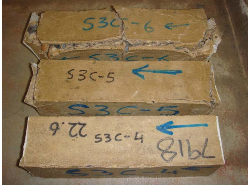
Plate 1 Failure of S3C (w/c 0.65) prisms after 570 days in 5% Na 2 SO 4 at pH 7
