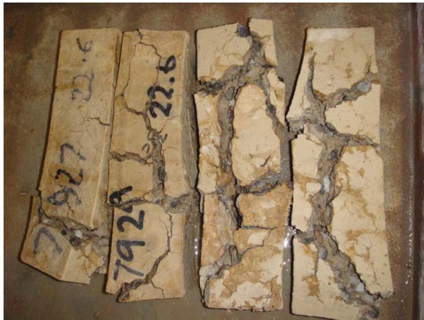
Plate 2 Failure of S3C (w/c 0.65) prisms after 570 days in 5% Na 2 SO 4 at pH 3.5
