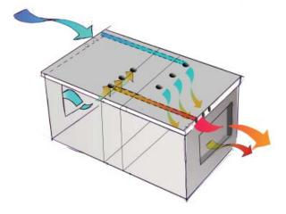
According to Chris Arkins, Director of ESD consulting firm Steensen Varming, "ventilating the slab in this way allowed absorbed heat to be purged overnight, enabling it to absorb heat during the day and provide passive cooling to the spaces. The key outcome achieved was to allow cross ventilation to the bedrooms without compromising privacy."
