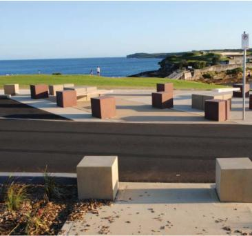
The highly corrosive coastal environment created by salt spray required careful consideration of materials, with concrete the obvious choice in terms of its impressive durability and minimal maintenance. The choice was the use of nearly 600 elements in five different shapes - wheel stops, separation blocks, kerbs and two styles of bollards that provided a 'garrison look' to the project.
